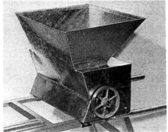
Completed hood-and-hopper assembly is riveted throughout. Note that the tabs of the hopper's upper edge are folded flat to eliminate the sharp edges
