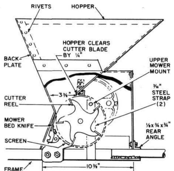
panded-metal screen (preferably heavier) 16 in. long and as wide as the mower bed-16-1/2 in. in this case. Pass it over the reel, under the mower bar and keep it close around and under the reel. Then bring it up inside and snug against the bed. Drill for 1/4 x 3/4-in. stove bolts at the ends of the bed where they will not interfere with the reel, and attach the screening.
