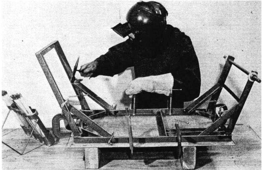
Sturdy carriage for the mulchmaker is completely welded: The board to which the frame is clamped to prevent warping is insulated from the table
