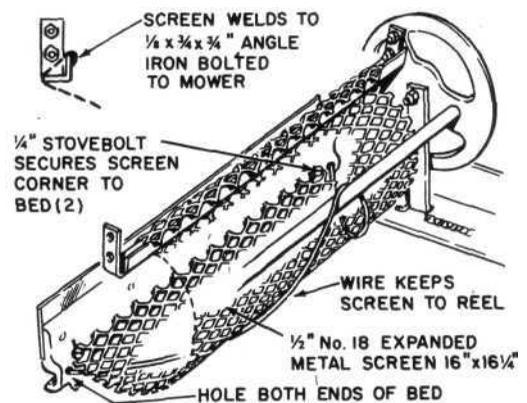
Screened reel produces a finer mulch and covers the whirling blades underneath. With the help of the retaining wire, the screen is a close fit; it serves as additional bed knives
