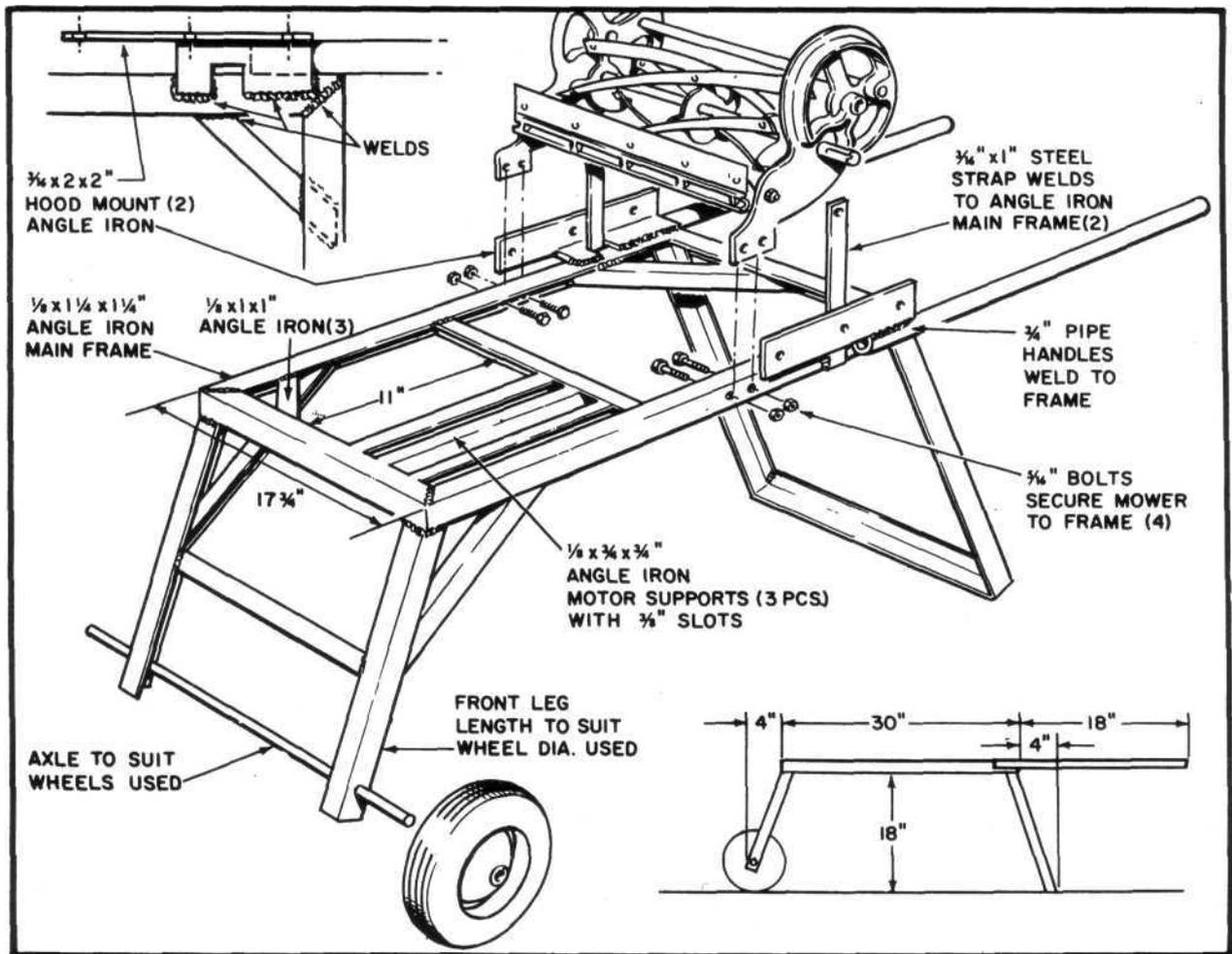
illustrations here if a 16-in. mower is used. The width would have to be varied for any other size mower.
