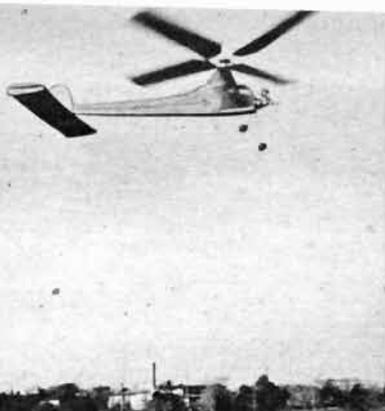
**LAUNCH MODEL** with the rotor blades spinning rapidly; use gentle forward motion.
