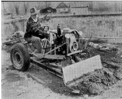
**Homemade bulldozer** attachment hangs on rear axle of tractor. As the sketch shows, Matous
